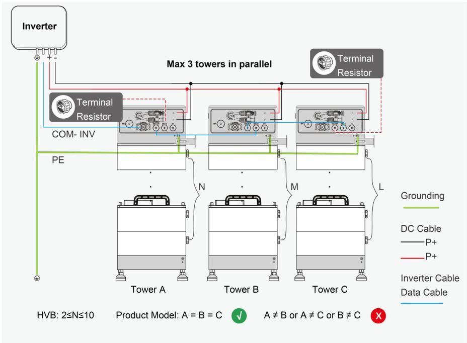
When multiple battery systems work in parallel, terminal resistors must be installed:
